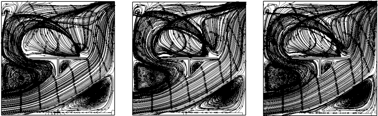
Figure IV.16 : Temperature contours (a) and streamlines (b) for different Pr numbers ( Re = 500 , Ri = 1 , K = 1 ).
