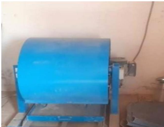
Photo III-5: La machine Los Angeles [17]
