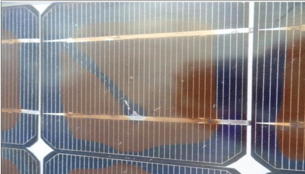
Figure III.19 : Fissure de la cellule
