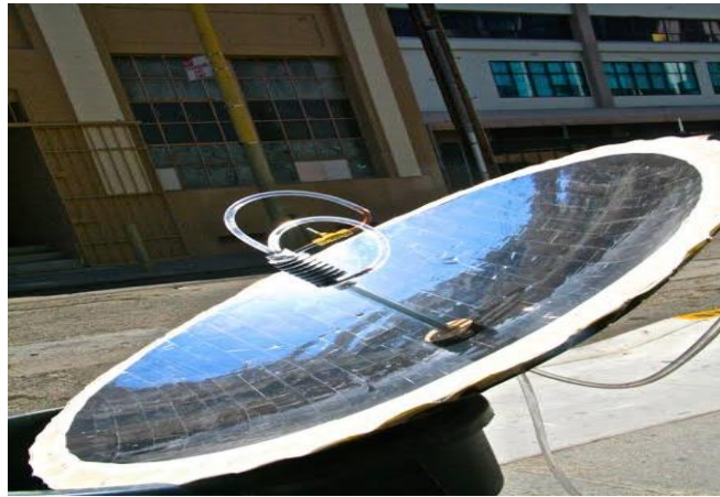
Figure 9 : Solar water heater [21]
