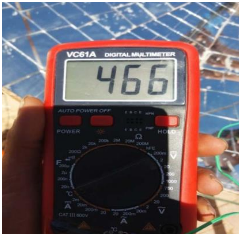
Figure 21 : Photo of the digital multimeter used (VCA61A - LCD)
