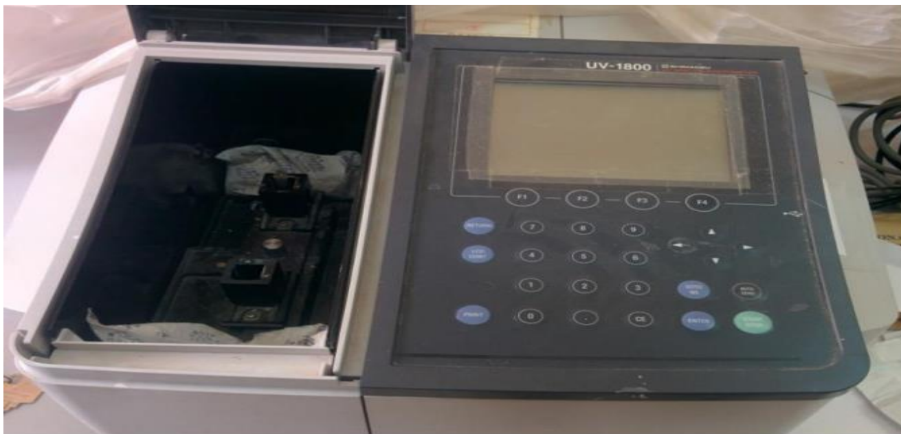
Figure 27 : Experimental UV-visible spectroscopy device UV-1800 used
