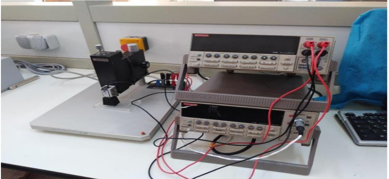
Figure 31 : Experimental setup of device of the Four-Probe Method used (KEITHLEY 2400)
