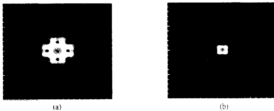
Figure 4.5: the distribution of field intensity for a PCF with tetragonal lattice at 1.55 \mu\text{m} wavelength: (a) with air hole diameters of 0.8 \mu\text{m} . (b) with air holes diameter of 2.8 \mu\text{m}
