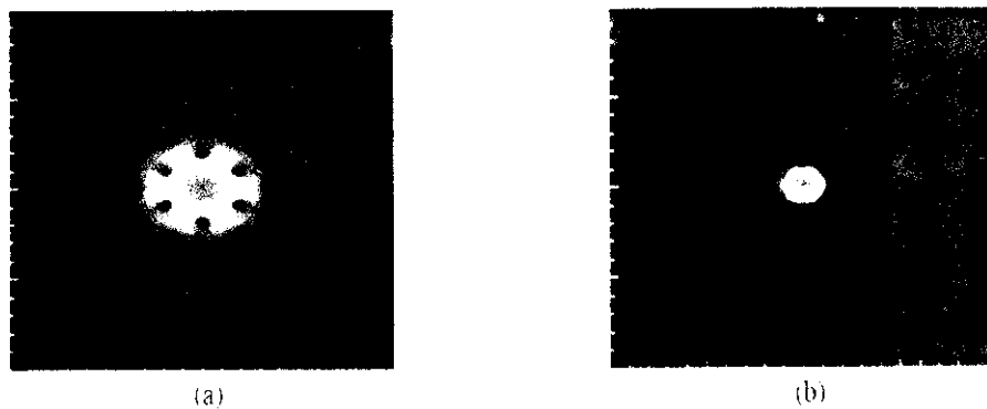
Figure 4.4: the distribution of field intensity for a PCF with triangular lattice at 1.55 \mu\text{m} wavelength (a) with air hole diameters of 0.8 \mu\text{m} . (b) with air holes diameter of 2.8 \mu\text{m}
