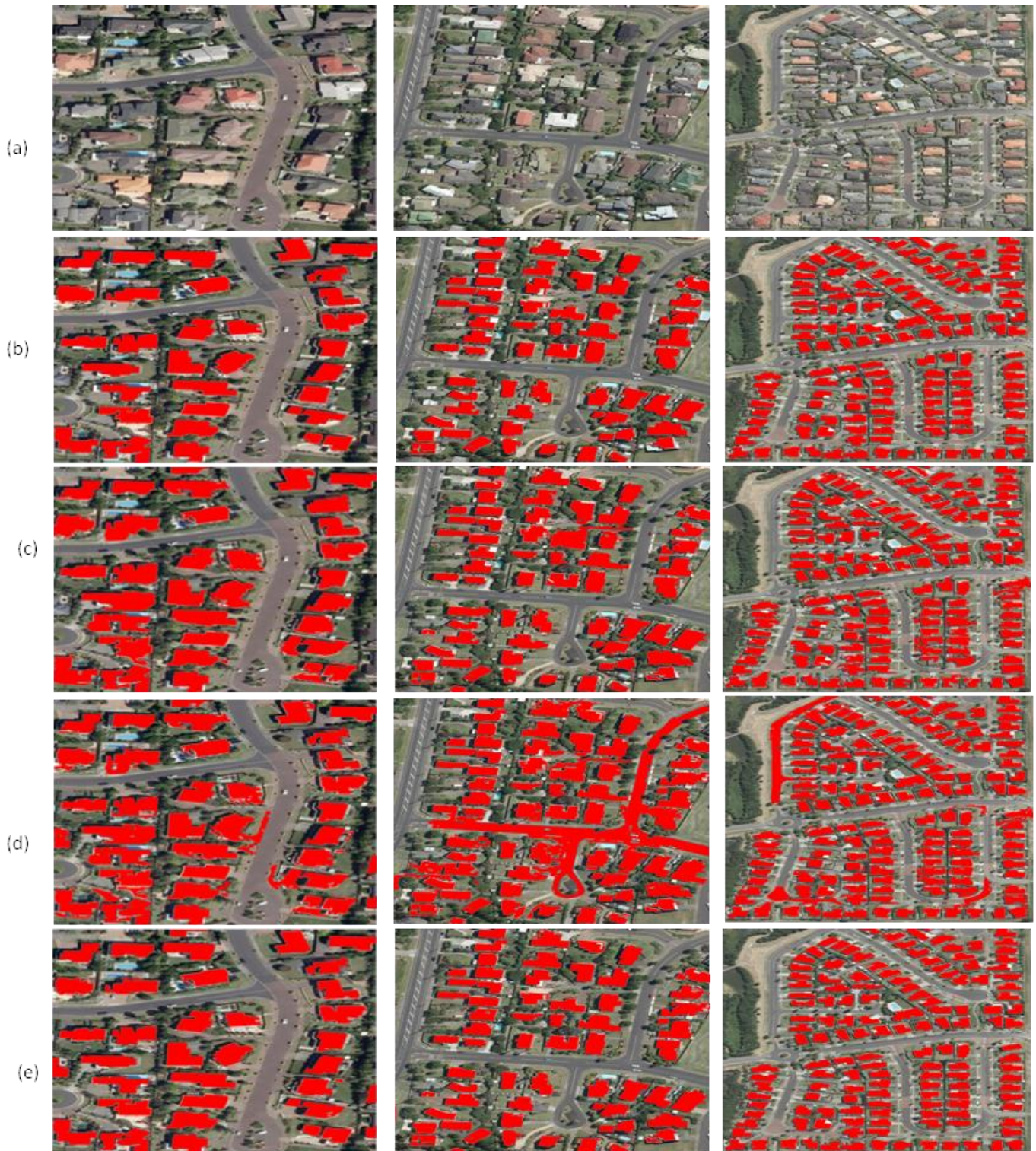
Figure 5.5: comparing the findings of three distinct algorithms for building recognition (row a) input images, (row b) The outcomes of the suggested technique, (row c) The method's outcomes of (Zhang et al., 2020), (row d) The method's outcomes of (Chen, Shang and Wu, 2014) and (row e) The method's outcomes of (Lv et al., 2016). (Red signifies building) .
