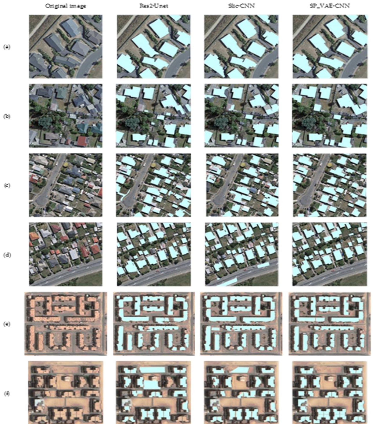
Figure 5.13: Optical evaluation of aerial images dataset segmentation. Column 1 designates the original image, column 2 is the outcome of Res2-Unet (Chen et al., 2022); column 3 is the outcome of SLIC-CNN; column 4 is the outcome of our proposed method SP_VAE-CNN, (a,b) are examples from WHU images 2016 dataset, (c,d) are examples from New Zealand imagery of Masterton; (e,f) are examples from high-resolution Google Earth images.
