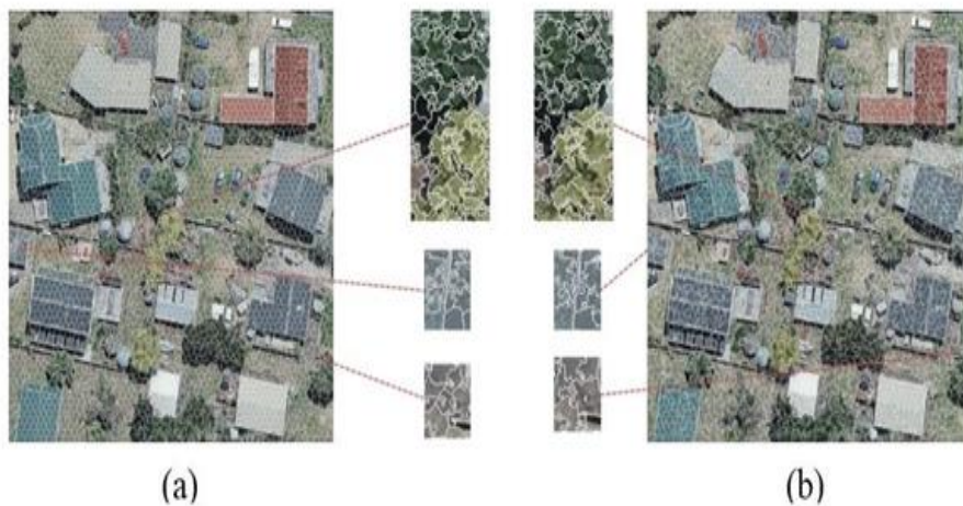
Figure 5.8: Outcomes of SLIC segmentation; (a) with a five-dimensional vector [l, a, b, x, y]; (b) with an eight-dimensional vector [l, a, b, e, h, c, x, y].
