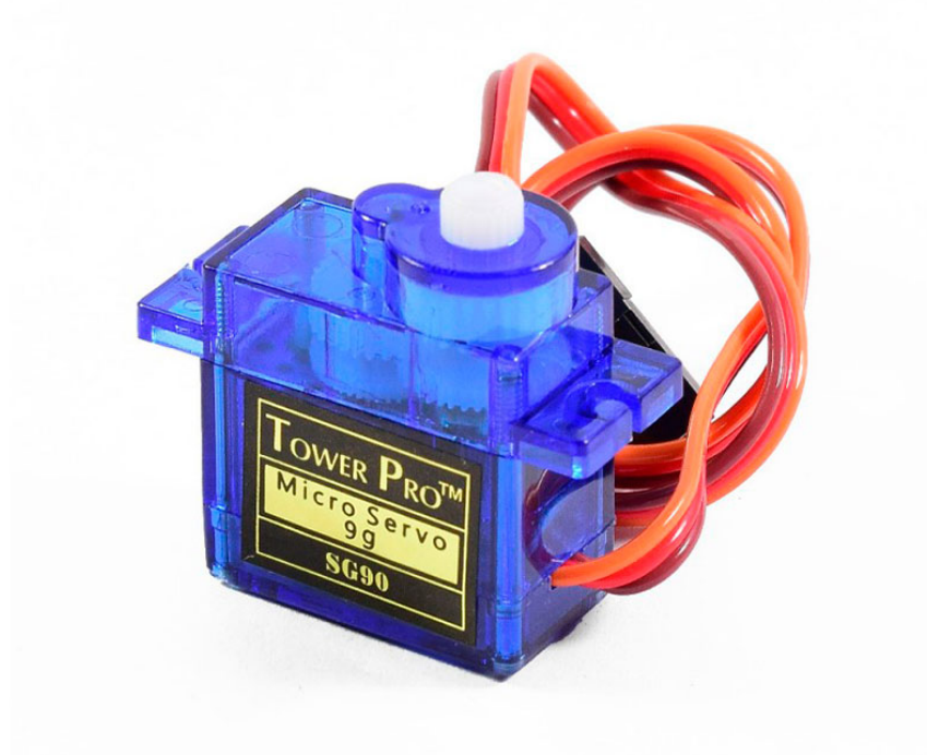
Figure 2.11: Servo motor SG90
