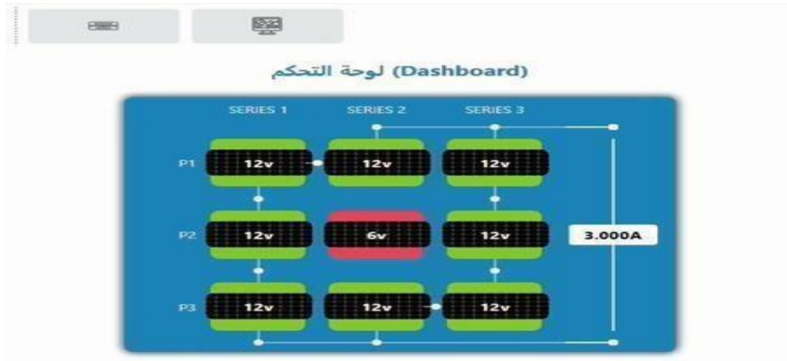
Figure 4.7. Connecting the panel array in case of failure on the HMI interface
