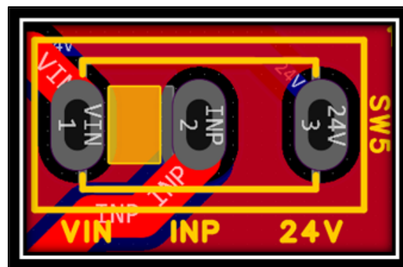
Figure 3.7. Battery switch design
