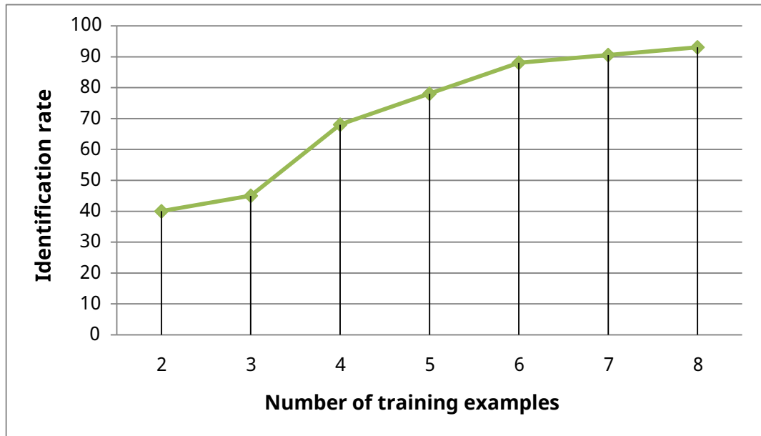
Fig.IV.11:Identification rate depending on the number of learning examples per person (ACP).
