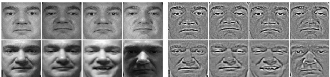
Fig.III.15: Illustration of the application of the proposed illumination correction method by Tan and Triggs.
