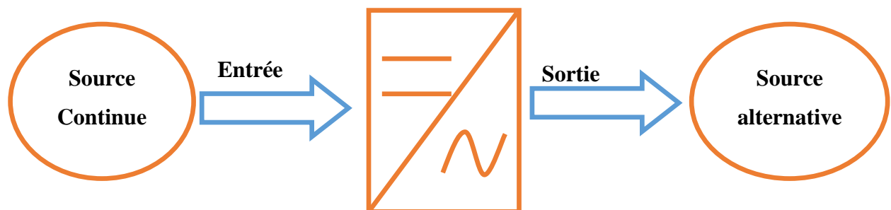
Figure I- 1 :Principe de la conversion Continu - Alternative (DC – AC)
