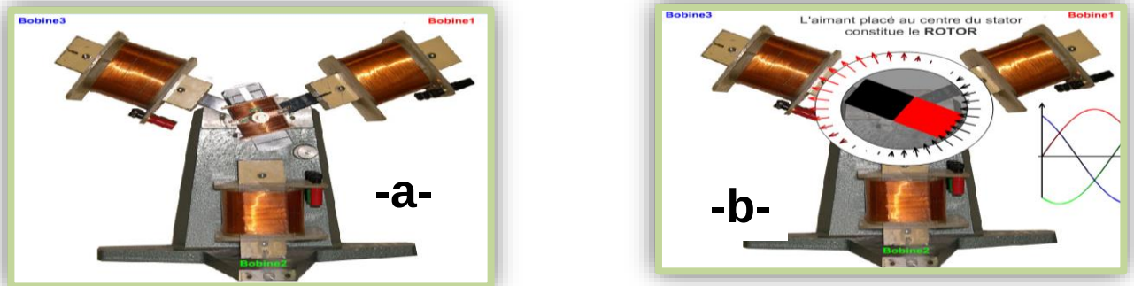
Figure IV.6 : (a) Wound-Rotor / (b) Permanent Magnet Rotor
