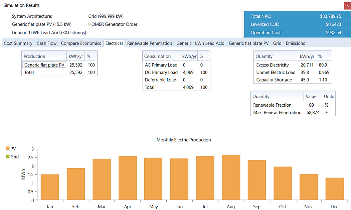
Figure 12: Electrical metrics for the 30kWh Lead-Acid system under total autonomy
