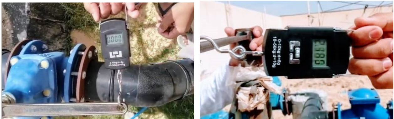
Figure III.1 Measuring Torque with a Digital Force Gauge
