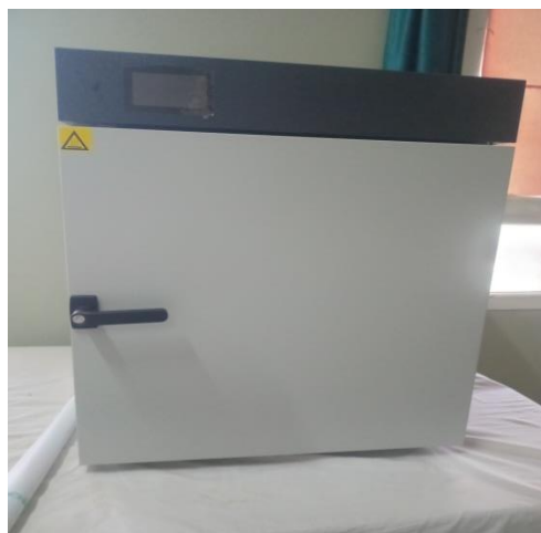
Drying oven (Personal photo)
