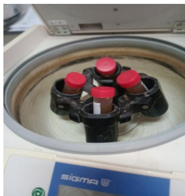
Figure 39: Centrifugal extraction.( Benchaoui S ; Hamidi A:2025)
