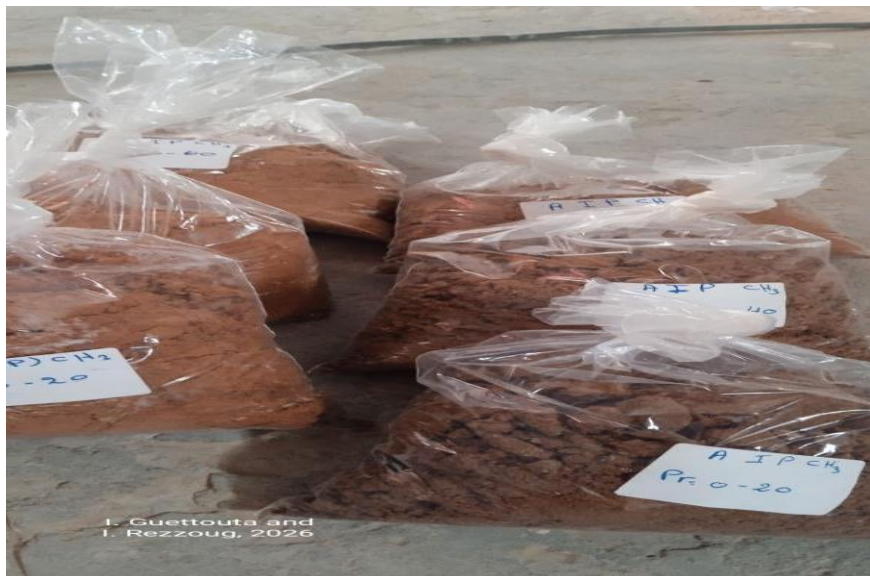
Figure (7): labeling, storage and preservation Soil sample
