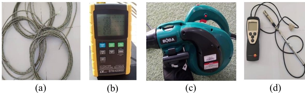
Figure II.3: Devices used in experimentation: (a) K-type thermocouple, (b) temperature digital recorder, (c) blower, (d) anemometer.
