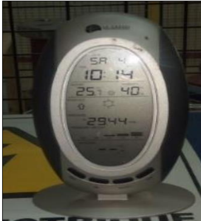
Figure III.6. Measurement instrument for atmospheric conditions (humidity, temperature, and pressure).
