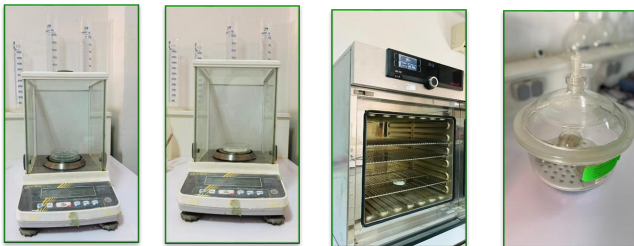
Figure 9: Experimental steps and equipment used for moisture determination (Original photos).
