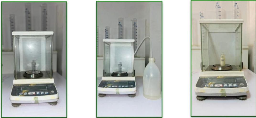
Figure 10: Experimental steps and equipment used for density determination (Original photos).
