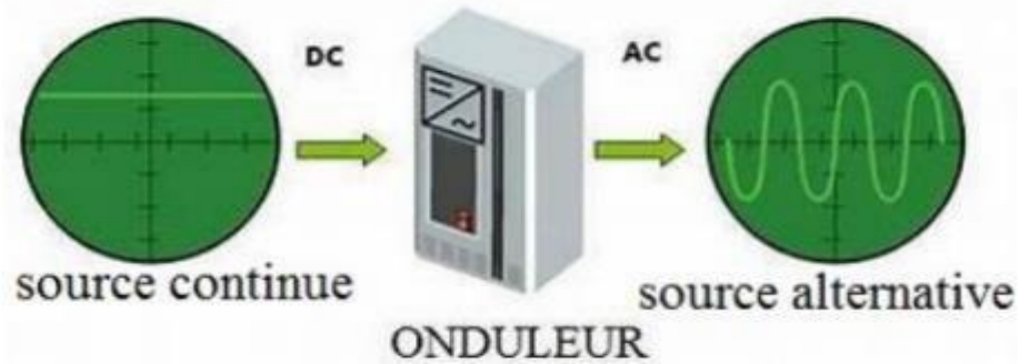
Figure II.23. Schéma de principe de la conversion Continu - Alternative (DC – AC)
