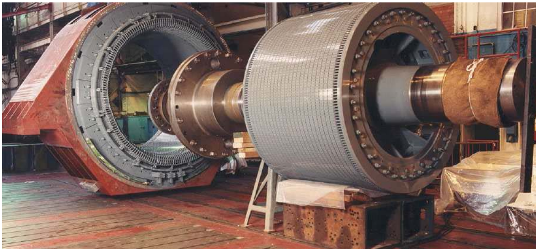
Figure 1.6: Machine asynchrone de 4.7 MW, 45tr/mn [5].
