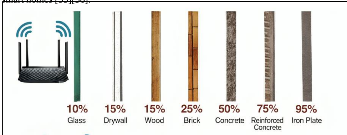
Figure I.20: RF attenuation caused by walls and indoor obstacles.
