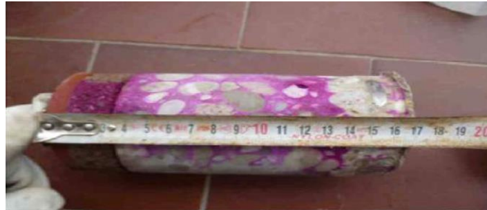
Figure II .9 : Test a la carbonatation
