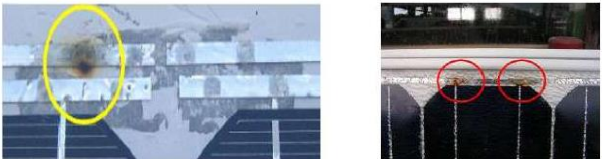
Figure (III.11): Increase in R_s Resistance Fault
