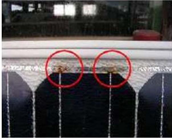
Figure II.29: Increasing series resistance fault .
