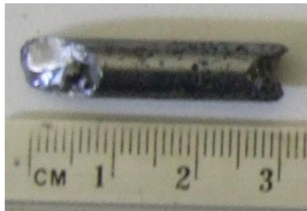
Fig.2. \text{CuIn}_{0.7}\text{Ga}_{0.3}\text{Se}_2 Sample showing complete solidification and good morphology
