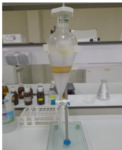
Figure III-7: The mixture (glycerol with biodiesel) in the separator for 24 hours
