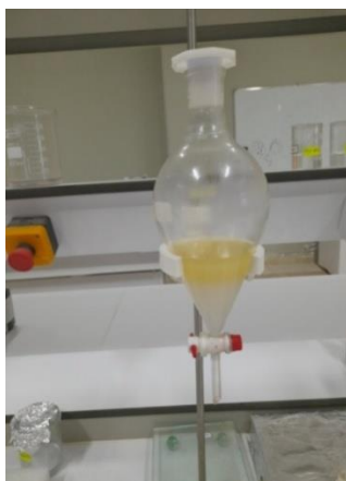
Figure III-10: The mixture (glycerol with biodiesel) in the separator for 24 hours
