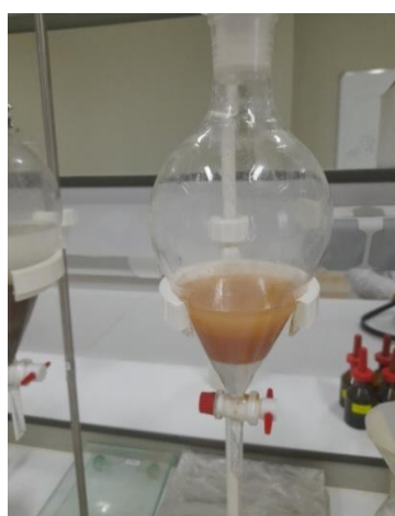
Figure III-9: The mixture (glycerol with biodiesel) in the separator for 24 hours
