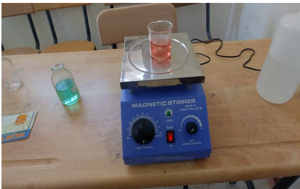
Figure III.6: The dopant and Stirring process
