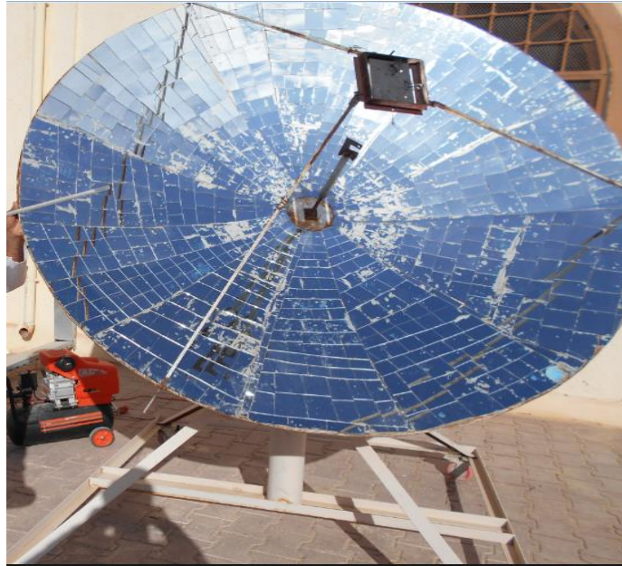
Figure I.16: General view of the solar concentrator used (laboratory22, Echahid Hamma Lakhdar University, El Oued).
