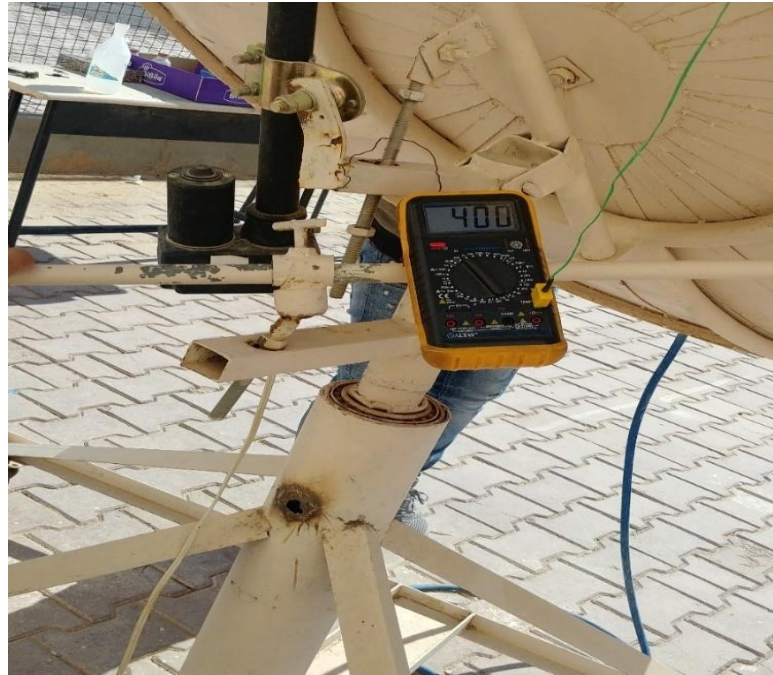
Figure III.8: The temperature used to heat the substrate (400 C°)
