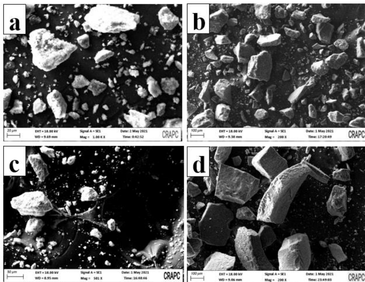
Figure IV.10 SEM images of NONPs biosynthesized using Punica granatum L peel extract at different molarities: (a) 0.01M; (b) 0.025M; (c) 0.05M; and (d) 0.075 M.
