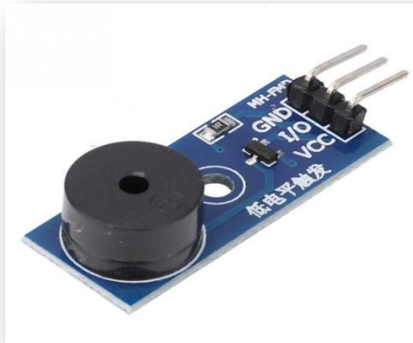
Figure II.10: "Buzzer" sound module
