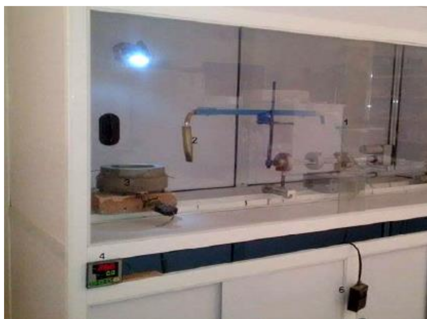
Fig. 3. 2. The deposition system of spray pyrolysis.
