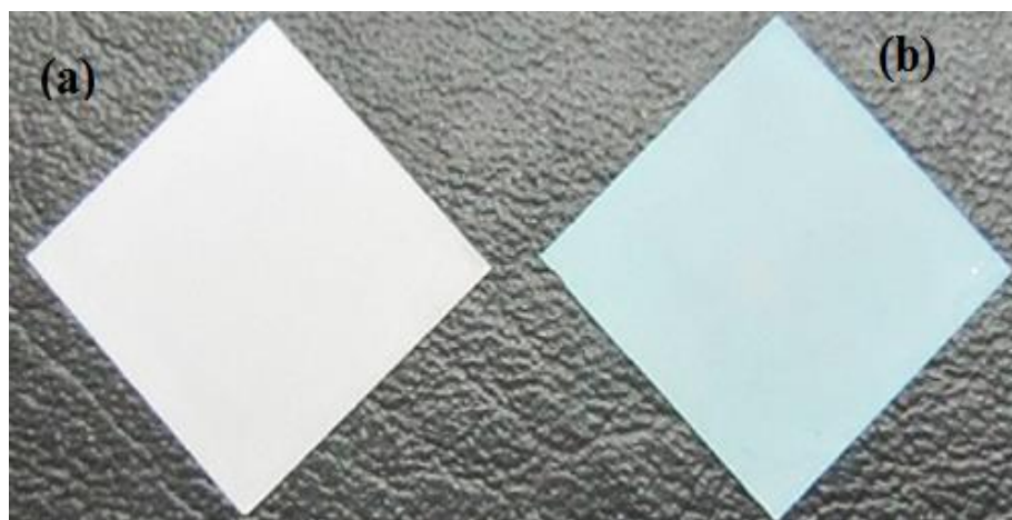
Fig. 4. 2. Photograph of ZnO/glass slide: (a) before and (b) after adsorption of copper ions .
