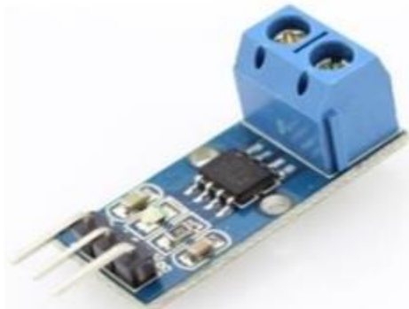
Figure.III.11: Current sensor Board module, Circuits.
