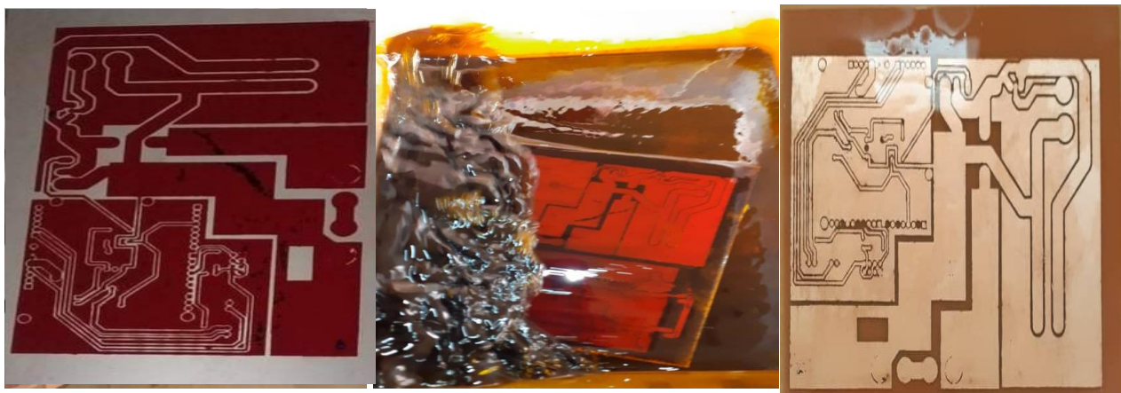
Figure.III.13: Stages of developing a printed circuit board (PCB).
