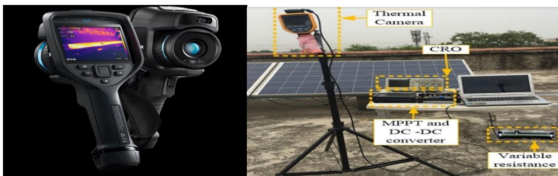
Figure I.40: Experimental setup at rooftop.[44]
