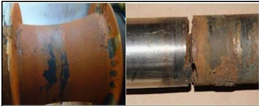
Figure III.10: Photos de la fatigue-corrosion
