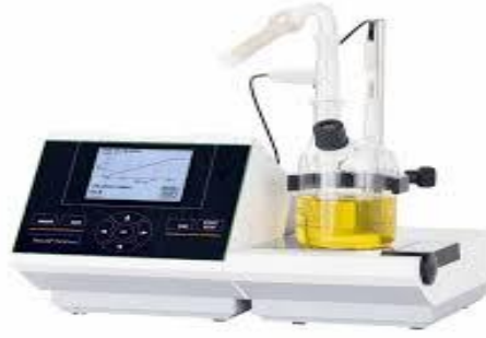
Figure II.1 — Water content measurement device (Karl Fischer titration unit).
