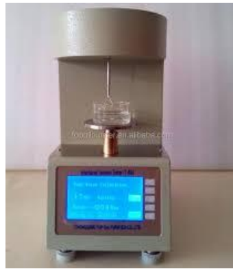
Figure II.5 — Interfacial tension measurement device (ring method, ASTM D971).
