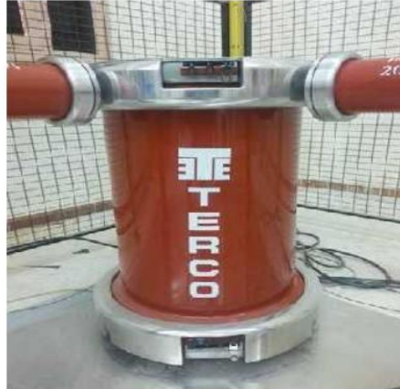
Figure III.2 — High Voltage Transformer 15 kVA high voltage test transformer
