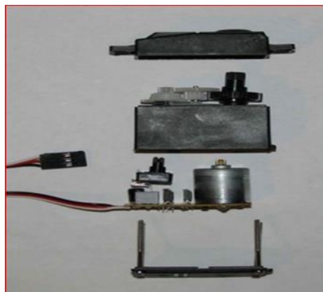
Figure II.7: A dismantled view of the larger Servo motor
