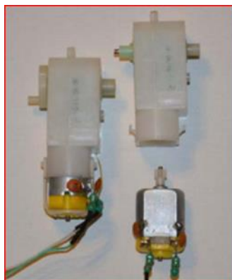
Figure II. 6: Here you can see a small DC gear motor (left) and again with the DC motor removed from the plastic gear box.
