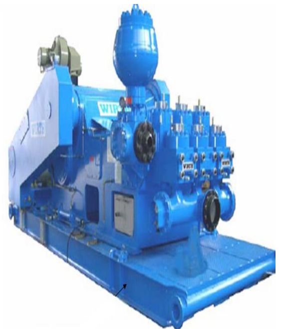
Figure II.13 pompes de forage
