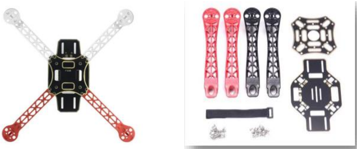
Figure (III.7) : Châssis quadrotor F450
