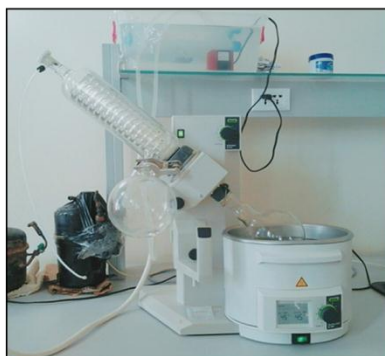
Figure 02: Evaporateur de type Rotavapor BUCHI Haeting bath R-491 (photo originale)
