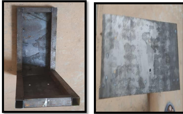
Figure III. 5 Soudage du support métallique
