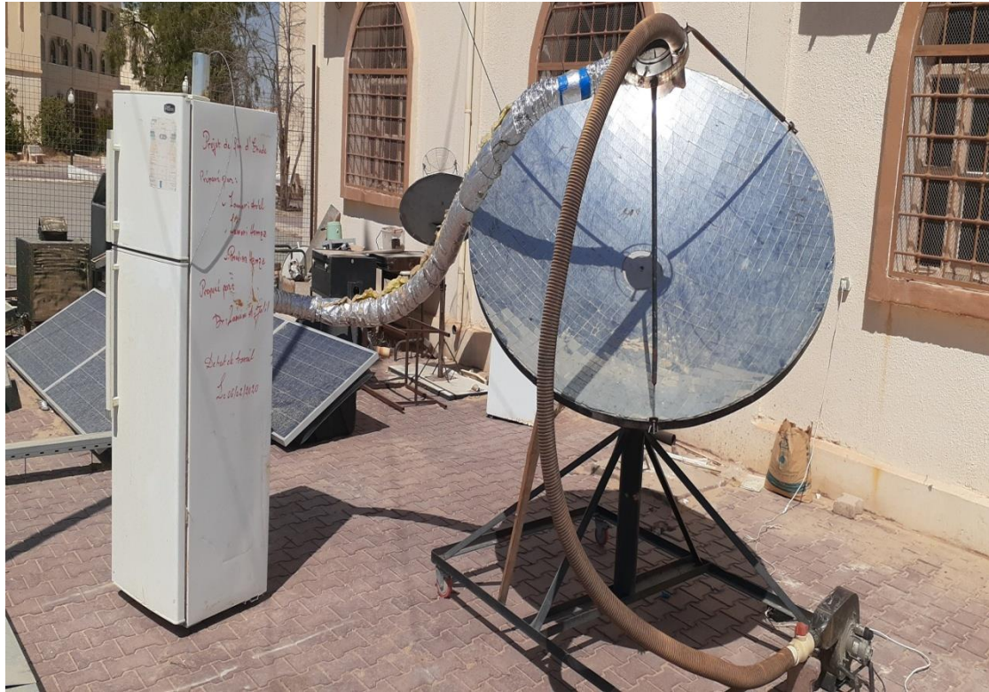
Figure III.4: model of the forced convection indirect solar dryer used
