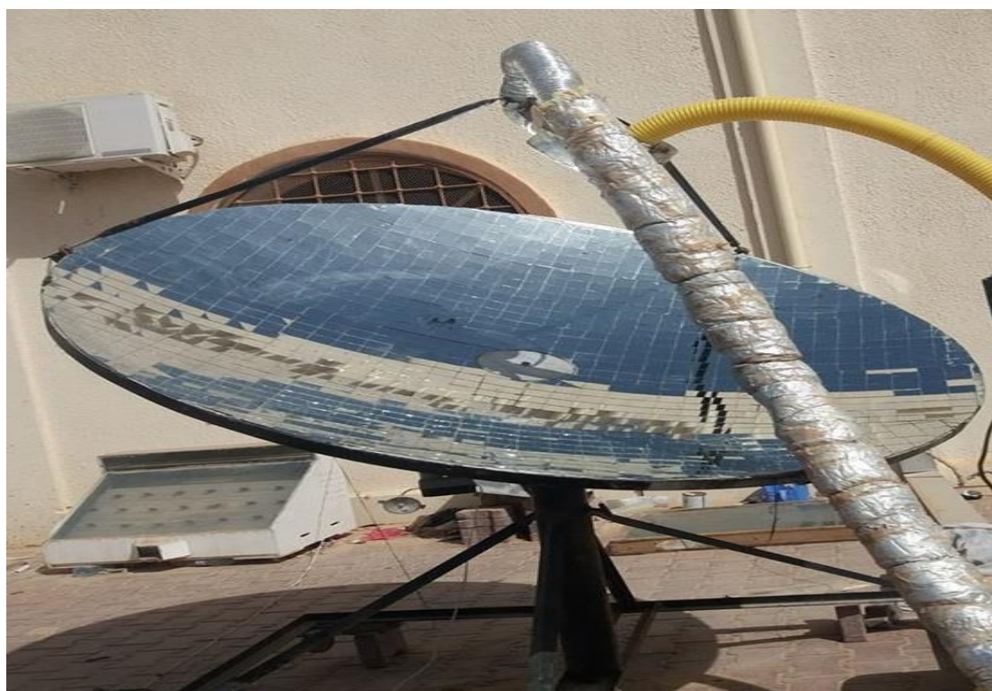
Figure III.1: Solar air collector.
