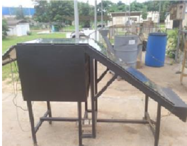
Figure I-3: Prototype De Séchoir Solaireactif Indirect [5]
