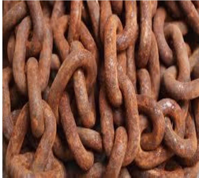
Figure 1.3: Metal affected by uniform corrosion.
