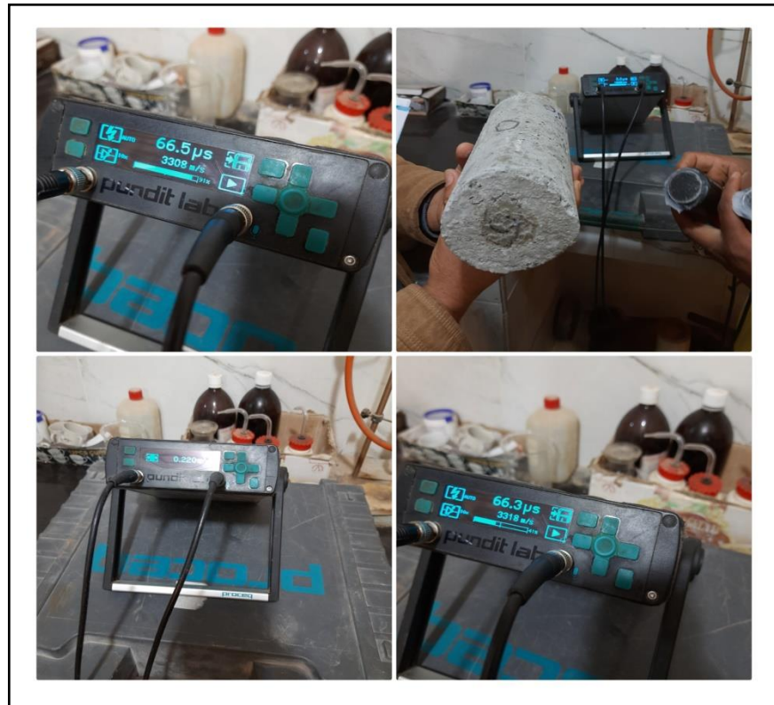
Photo III-08: Appareil de test ultrasonique Pundit-Lab
