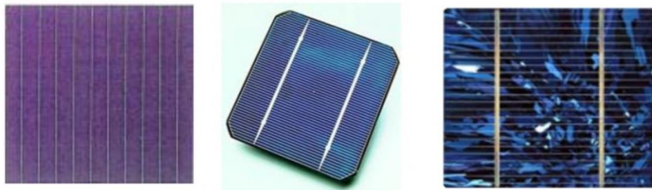
(a) Cellule amorphe (b) Cellule monocristalline (c) Cellule poly-cristalline
