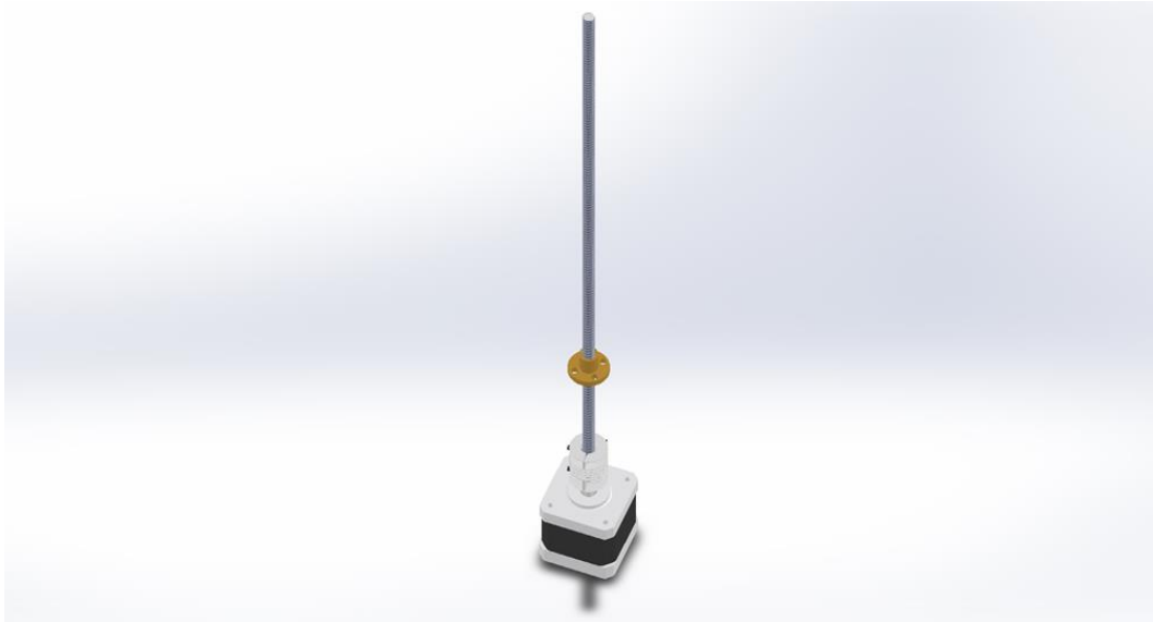
Figure IV.10: The Z axis motion transformation
