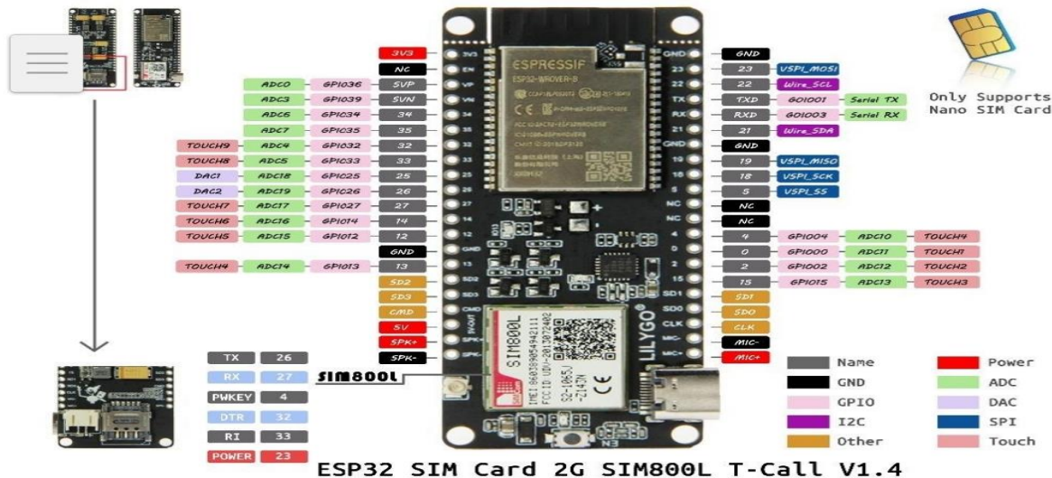
Fig III.8 TTGO T-Call esp32 sim800l card [5]
