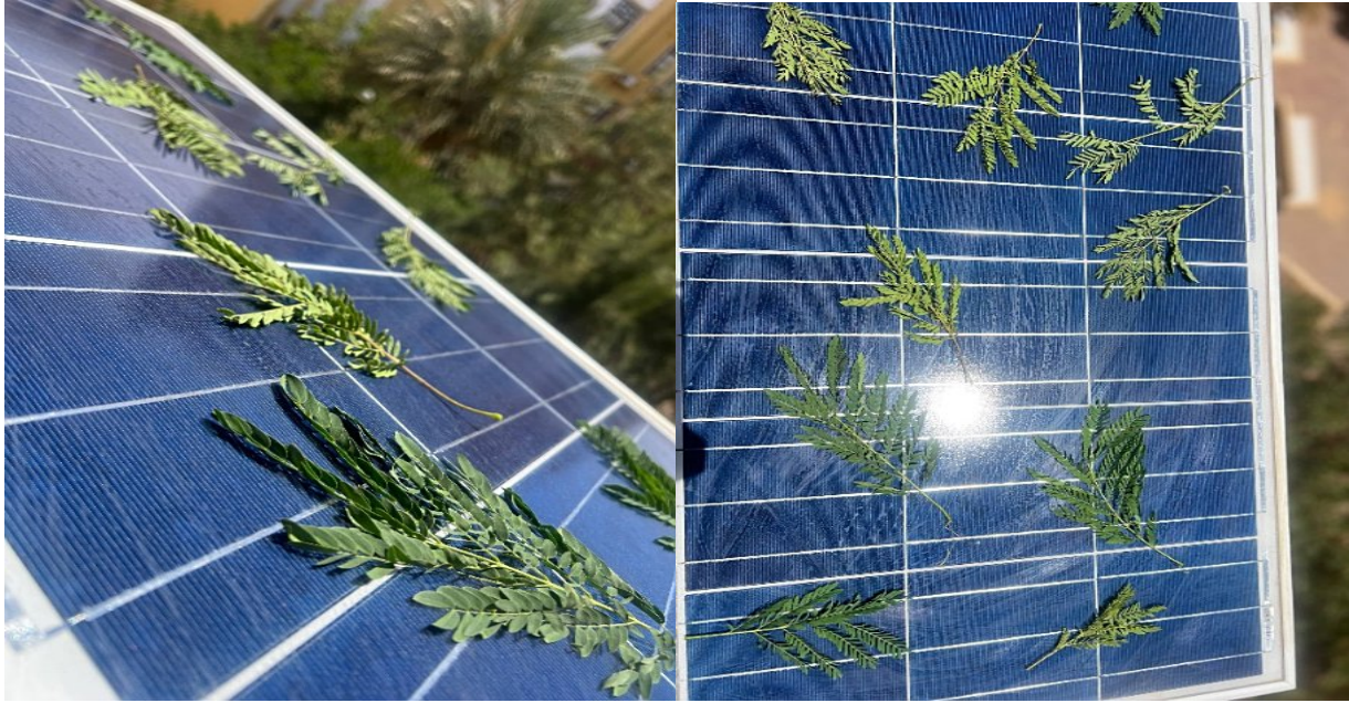
Figure 4.15:Measurement with a malfunction (dying the leaves)
