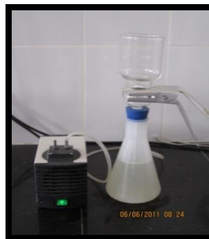
Figure III -5: montage de filtration.
