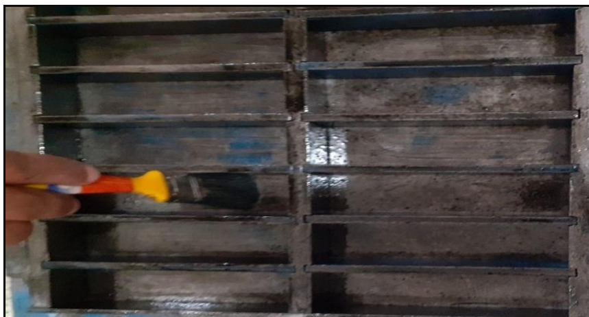
Figure III.8 : Lubrification des moules (4 \times 4 \times 16) cm 3
