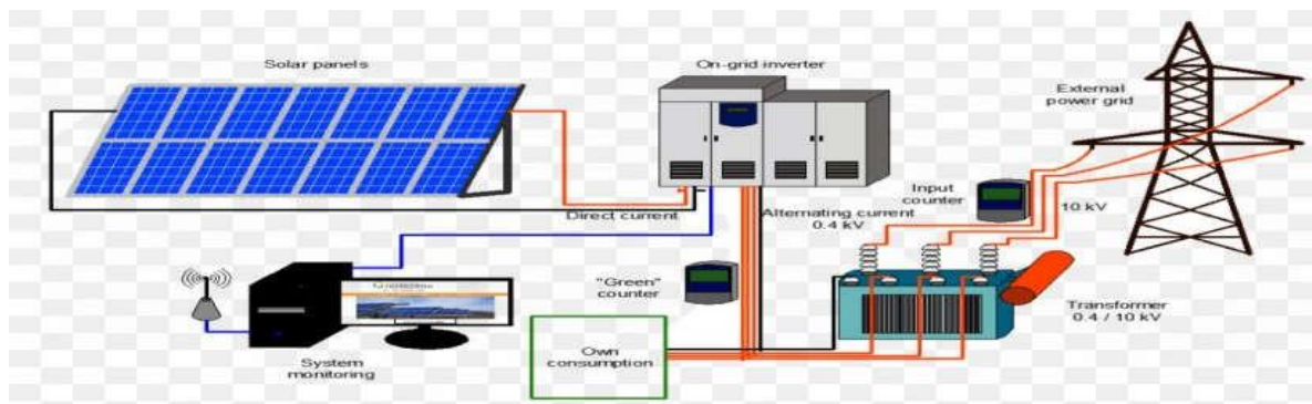
Figure I.14: Diagrammatic illustration of a PV system connected to the grid.
