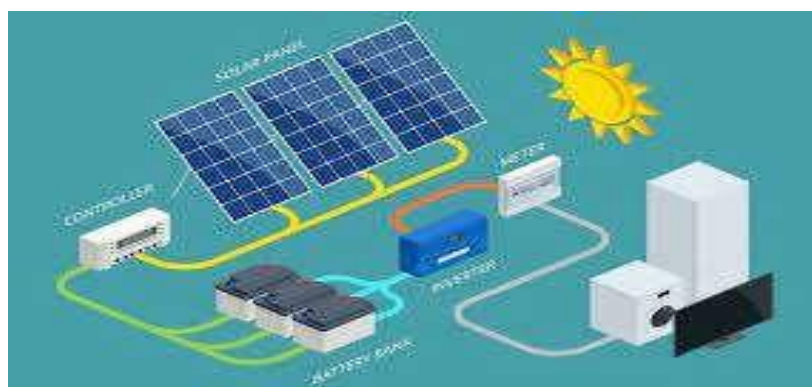
Figure I.27: An application of photovoltaic systems.
