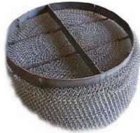
Figure III.7: Le Coalesceur ( Wire Mesh )
